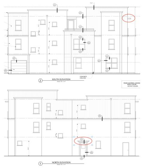
These appear to be 8" tall and project out a little under 2 feet. Given the ones on the West elevation are over juliette balconies and no one is standing under them for rain protection, I would assume some sort of aluminum louvered sunshade would work. Or a 2x8 perimeter frame with a perforated aluminum panel on top.
