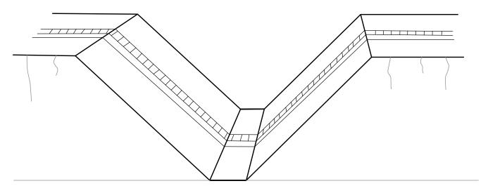
NOTE: ONE KEY TRENCH IS SUFFICIENT FOR DAMS UP TO 5 METERS HIGH. TWO OR MORE KEY TRENCHES ARE REQUIRED FOR DAMS OVER 5 METERS HIGH.
